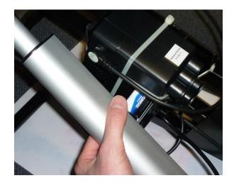
4. Push the two batteries back in to the compartment and reattach the battery compartment lid.
