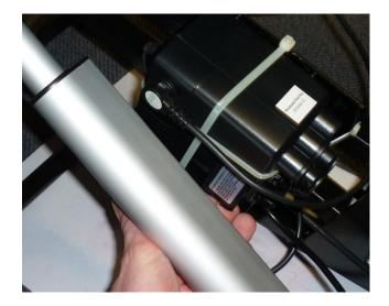
1. Raise the chair and lift up the fabric access flap at the rear to locate the control box. Using your finger nail, lift the locking tab on the bottom of the battery compartment lid and release.
