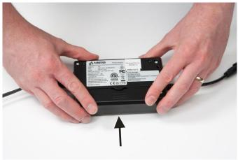
4. Slide the battery compartment lid back on to the power supply.
