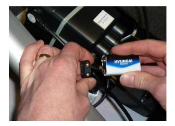
3. Connect two 9V batteries to the tab terminals pulled out from the battery compartment.
