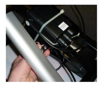
2. Reach in to the battery compartment and pull out the two battery tab terminals from the compartment.
