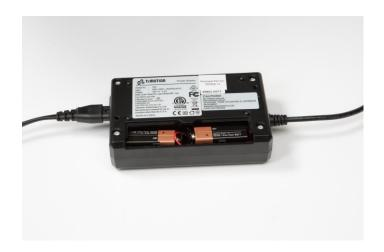
3. Place the batteries and wiring inside the battery compartment of the power supply.
