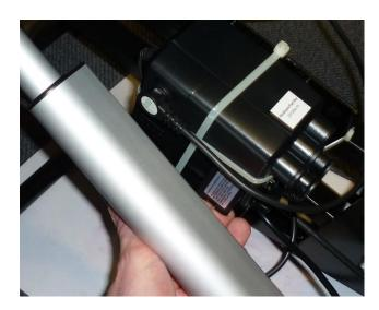
1. Raise the chair and lift up the fabric access flap at the rear to locate the control box. Using your finger nail, lift the locking tab on the bottom of the battery compartment lid and release.
