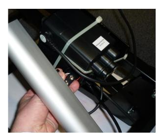
2. Reach in to the battery compartment and pull out the two battery tab terminals from the compartment.
