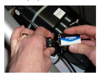
3. Connect two 9V batteries to the tab terminals pulled out from the battery compartment.
