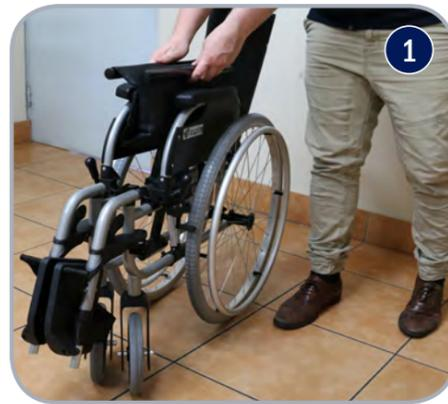
2. Pushdown on the side seat rails of the wheelchair until the seat is flat to unfold the frame
