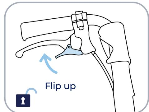
**UNLOCK:** To disengage brakes, flip the switch upwards.
