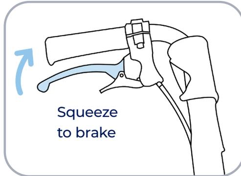
**BRAKE:** To engage brakes, squeeze the handbrake in an upwards direction.
