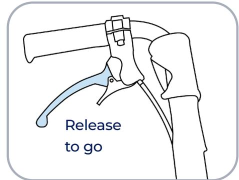
**RELEASE BRAKE:** To disengage brakes, release the handbrake.
