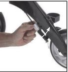
**WARNING:** Always test the brakes after adjustment. Ensure the brakes will safely slow down and hold the Rollator in the parked position.
