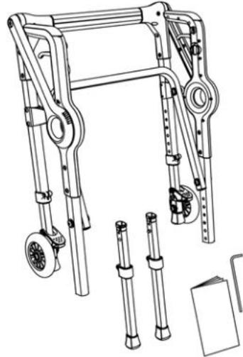
2.5mm Allen Key needed for assembly of the Roami PMA.
